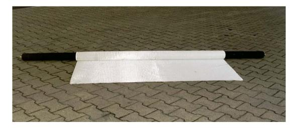
Outside is the tangled fibre layer clearly visible, this is important for a good bonding to the carrier pipe. Simultaneously, the other tangled fibre layer is facing the packer. This is important for a smooth moulding and a good resistance to high pressure flushing.
