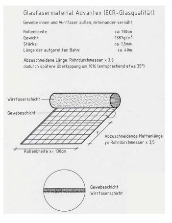
fibre glass matting can be installed in two or three layer form. Remembering the fibre glass matting are also of various area weight specifications. The RSV leaflet writes a minimum thickness of the liner to be of 3 mm. In the here attached test reports (see Annex 6.2) fibre glass mats of 1387g/m<sup>2</sup> area weight in two ply form were used. A data sheet for these mats can be found in Annex 6.1.1.
